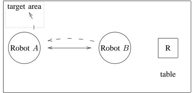
Fig. 1. Schematic figure of the environment. Solid arrows indicate movement of robots. Dashed arrows indicate movement of foam blocks. R is a realignment block. For a description of the realignment block see Section IV-C.
