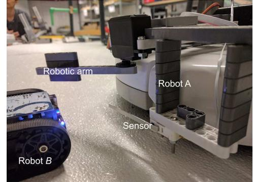
Fig. 2. Robot A in touch sensor configuration after successfully handing over the foam cube from robot B.
