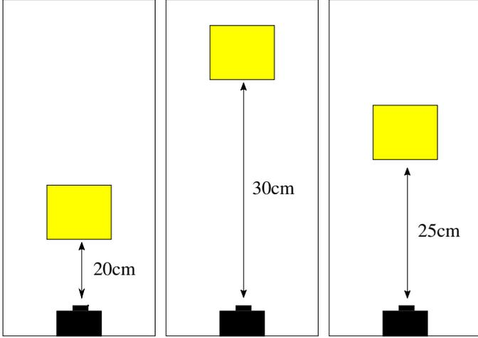
Fig. 6. Top view where the black boxes represent the camera and the yellow squares the 101.6 by 101.6 millimetre cube
