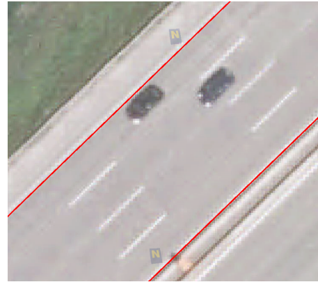
(b) Image after the Hough Line Transform using a threshold of 200 has been applied.
