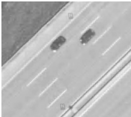
(a) Image filtered using the Gaussian Blur. The kernel size and \sigma are automatically calculated by OpenCV.
