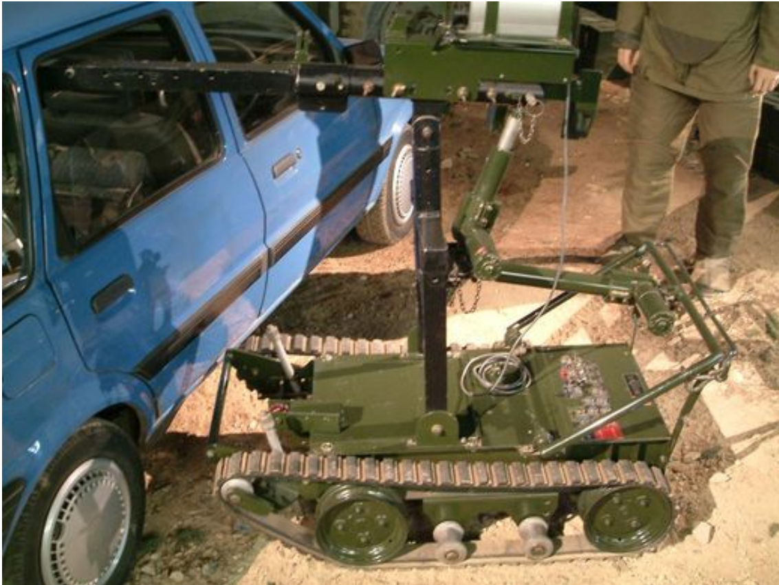
Figure 1.3: An early version of the Wheelbarrow bot with attached remote control cables 6 .
