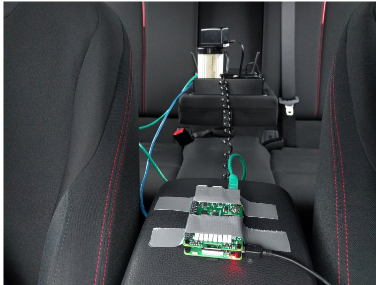
Figure 15.1: Car Mount of the Raspberry Pi accelerometer
