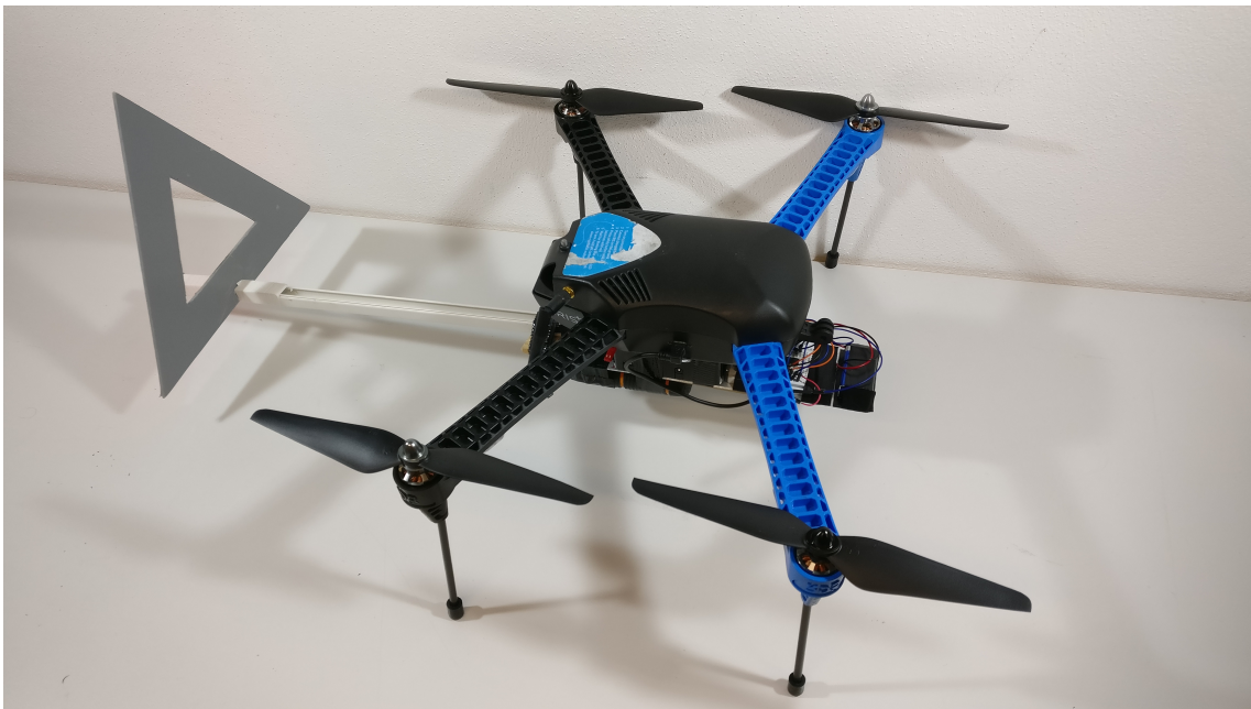
Figure 2.1: In this figure the 3DR Iris+ is shown with custom made breakdown triangle on a custom made control module attached to the main frame of the drone.
