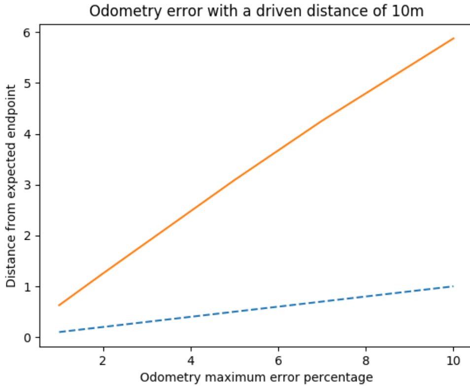
Figure 6.3: A figure representing the error of odometry for linear movement and a non linear movement. The dashed line represents the error for the linear movement whereas the solid line is the error of non-linear movement. The x-Axis represents the maximum percent and the y-Axis the maximum offset of the target distance of 10 meters.
