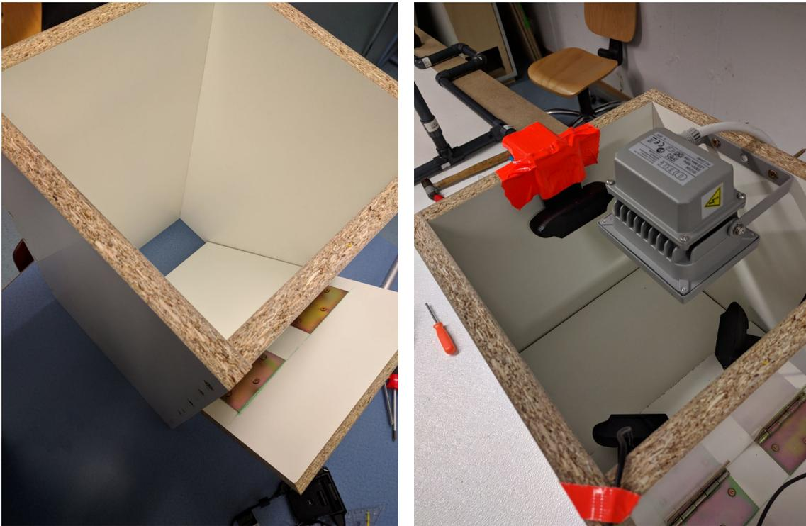
(a) Raw camera-box without cameras attached to it. (b) Camera-box with cameras and light attached to it.
