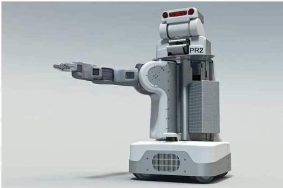
Figure 2.3: The PR2 with its spine at its minimal height and one arm raised
