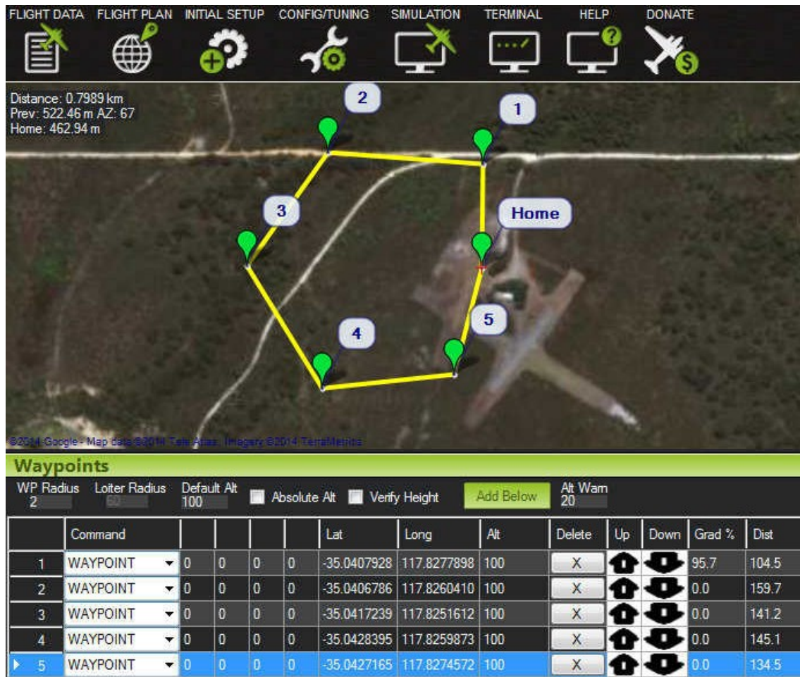
Figure 9.1: The Ground Control Station Mission Planner 3 . In the top window the user clicks on some points on the map to create waypoints for the drone. In the bottom all points are listed with their corresponding GPS coordinates and altitude.
