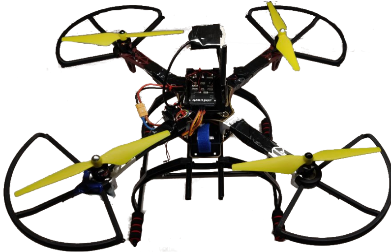
Figure 9.5: Image of the Drone used for the real world tests. It is equipped with 4 rotors, a flight controller placed in the middle of the frame and a gimbal mounted on the bottom connected to a companion computer used for processing images on the drone. The drone itself is a heavily modified Erle Copter 15 with a Pixhawk 16 flight controller.
