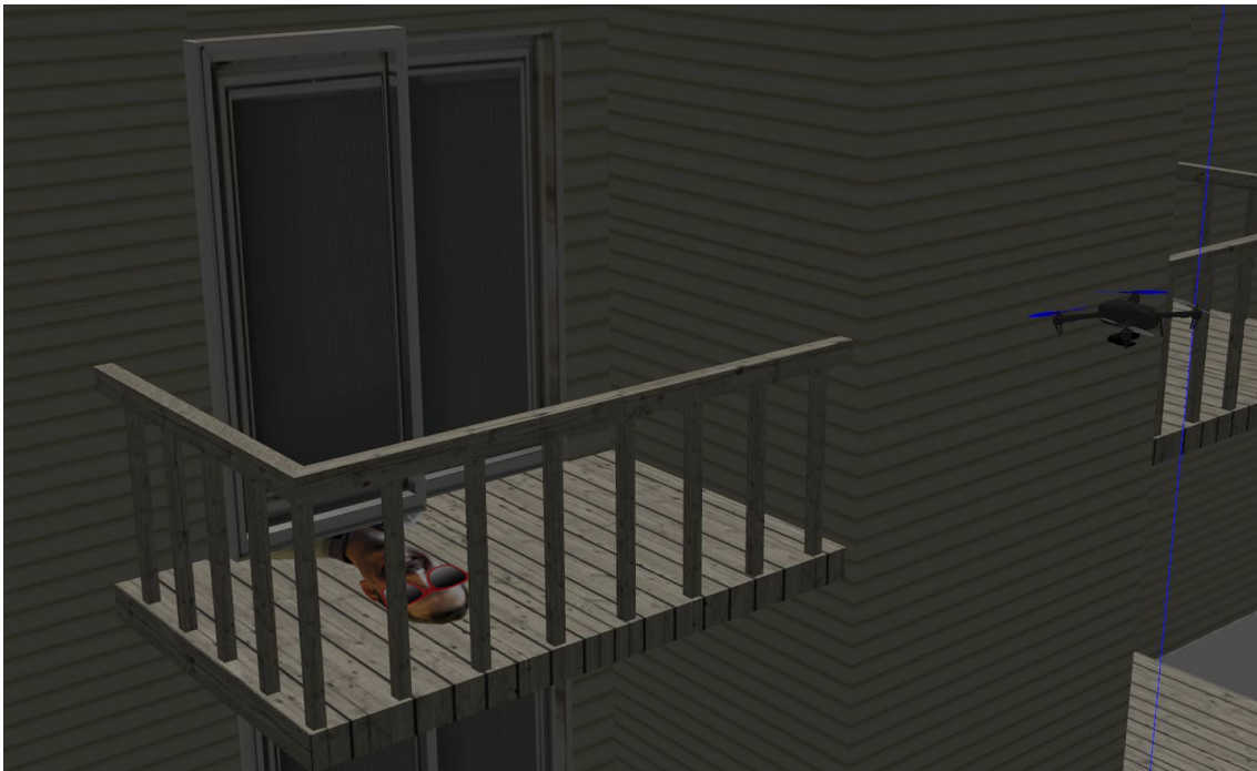
Figure 3.3: Shows the Gazebo simulator with our simulated drone looking at an apartment complex. A depth camera is mounted at the bottom of the vehicle providing data to ROS.
