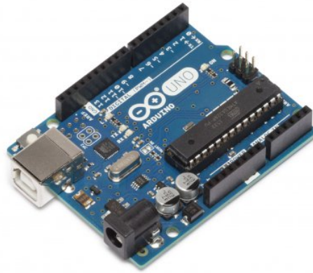
Figure 5.2: A picture of the Arduino Uno and its ports
