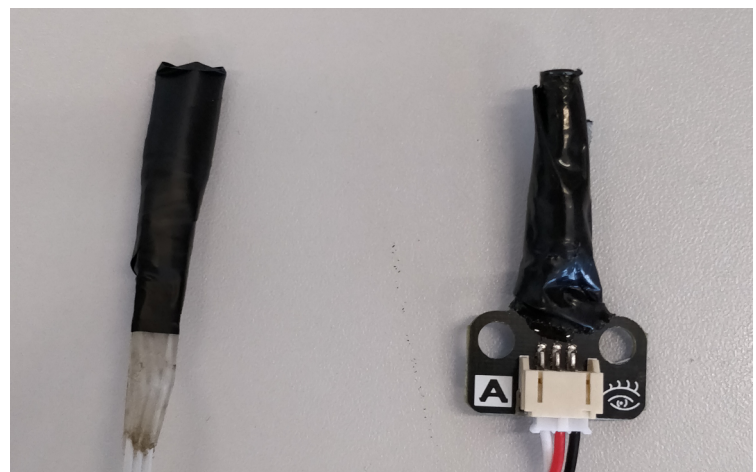
Fig. 2. The old light sensor on the left is missing the mounting board and attachment jack, while the new model on the right features both.
