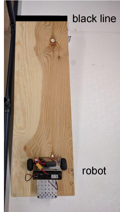
Fig. 1. Robot with the mass mounted at the front, in the starting position on the ramp. The black line indicates the top of the ramp.
