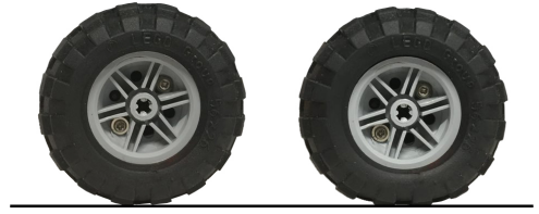
Fig. 4. Deformation of Tires. The left wheel carries only the weight of the metal base plate. The right wheel carries an additional mass, resulting in a bigger area touching the ground.
