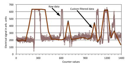
Figure 3 the shows difference а smoothing algorithm can make. The raw data come from an infrared distance-sensor. From the overall 1400 values this particular smoothing algorithm leaves all values that are out of tolerance of the previous ones. This results in an abstract view of the data without losing too much of the reasonable values.
